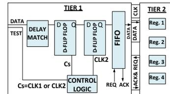
Figure 5. Loosely synchronous interface architecture for CDC in 3-D IC
