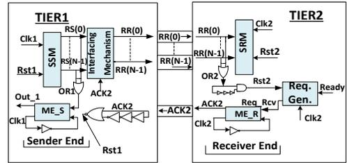
Figure 4. Architecture of QDI based GALS CDC technique in 3-D IC
